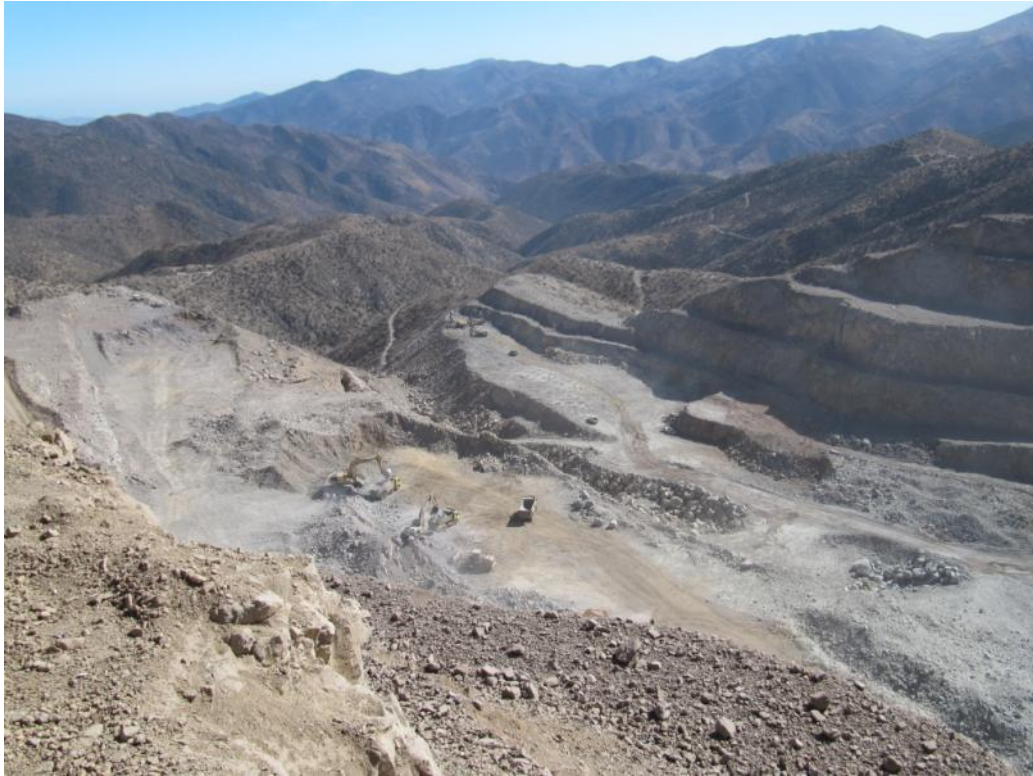
Figure 6 –Las Loas Pit –Pre Strip Completed to Final Pit Limit
